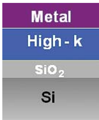
Schematic of a High-k, Metal Gate "Stack" with an SiO 2 Interfacial Layer
