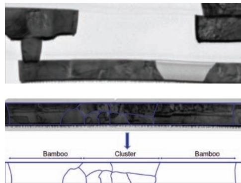
FIG.2A Void growth during electromigration
